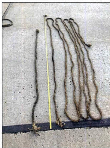
Figure 5. Stopper line displayed on the pier, approximately 83 feet, provided by Coast Guard Sector Delaware Bay Investigations.
