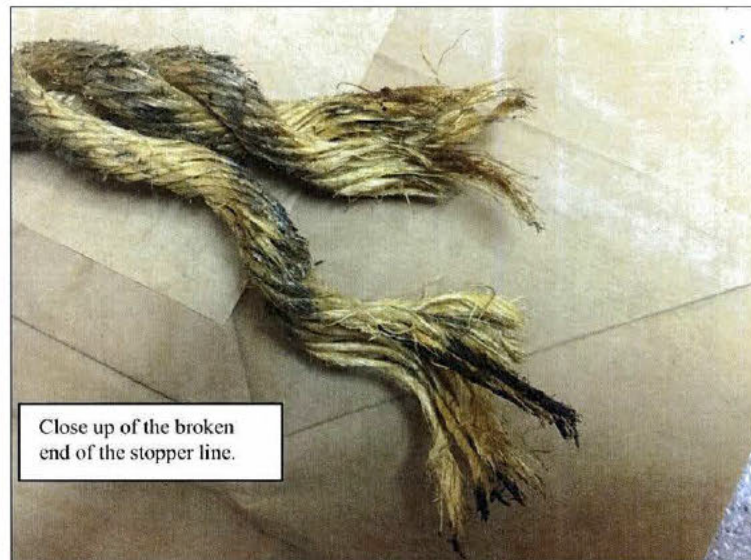
Figure 4. Stopper line broken end, provided by Mr. [REDACTED]
